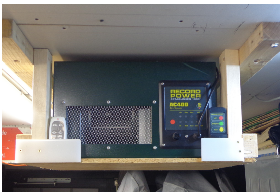
Record air cleaner fixed to the ceiling (the extraction & air cleaner remotes are in their storage "pockets")
